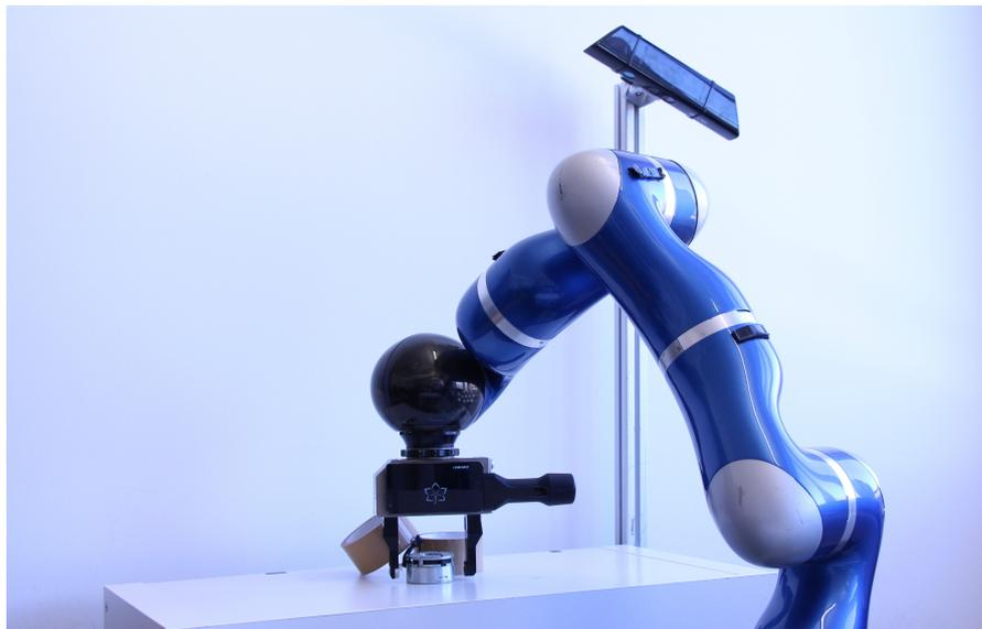
Figure A.1: Demonstrator setup with LWR-III, gripper, display and the kinect depth camera
